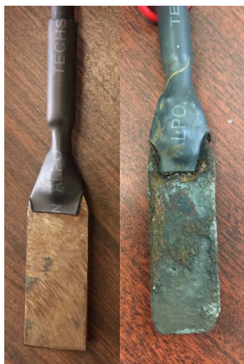
Figure 5: Bare Steel sample not encased in ConduDisc™ surround before (left) and after (right) the experiment.
