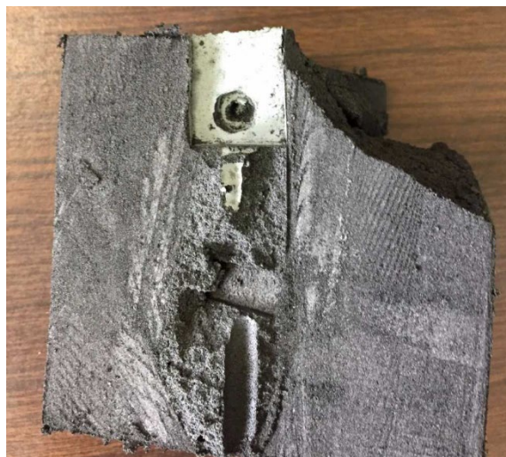
Figure 9: Cross-section of ConduDisc™ surround that had encased the galvanized steel plate sample
