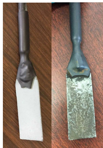
Figure 6: Galvanized sample not encased in ConduDisc™ surround before (left) and after (right) the experiment.
