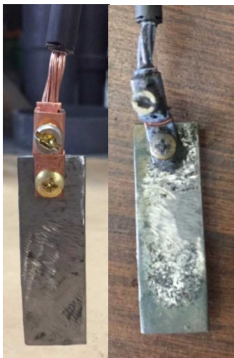
Figure 7: ConduDisc™ surround encased bare steel sample before (left) and after (right) the experiment.
