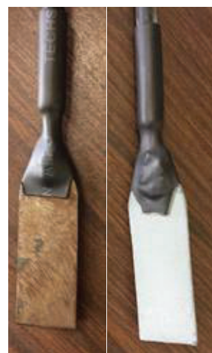
Figure 2: Samples made with shrink tube and soldered connection. (Bare Steel sample on left, Galvanized steel sample on right)
