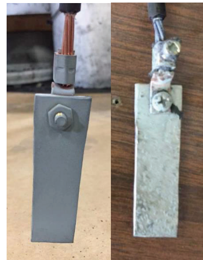
Figure 8: ConduDisc™ surround encased galvanized steel sample before (left) and after (right) the experiment.
