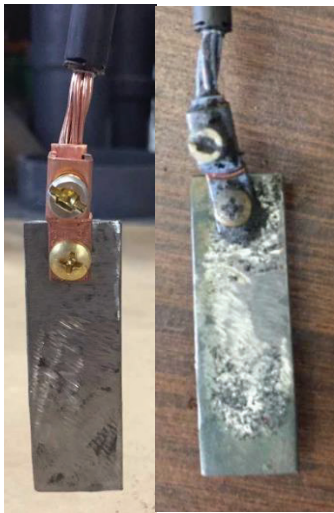
Figure 7: ConduDisc™ surround encased bare steel sample before (left) and after (right) the experiment.
