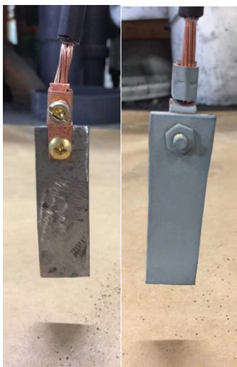
Figure 1: Samples made with mechanical lugs. (Bare Steel sample on left, Galvanized Steel sample on right)
