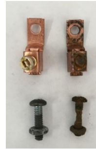
Figure 2: The Connection Hardware before (left) and after One Month of the Experiment (right)
