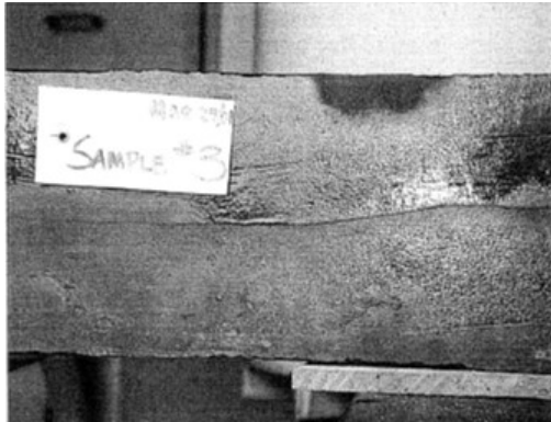
Figure 3: Crack in Wet ConduCrete Pro Electrode after Power System Fault Current
