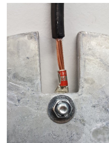
Figure 2: Copper Compression Connector Attachment to the Galvanized Steel Grounding Plate (left and middle) and the ConduDisc Inner Plate (right)
