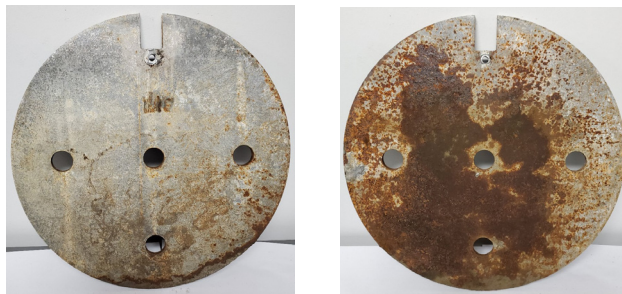
Figure 13: Galvanized Steel Grounding Plate, After Experiment
