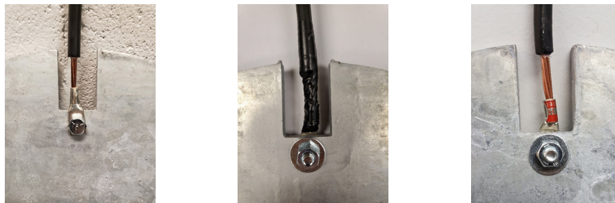
Figure 2: Copper Compression Connector Attachment to the Galvanized Steel Grounding Plate (left and middle) and the ConduDisc Inner Plate (right)
