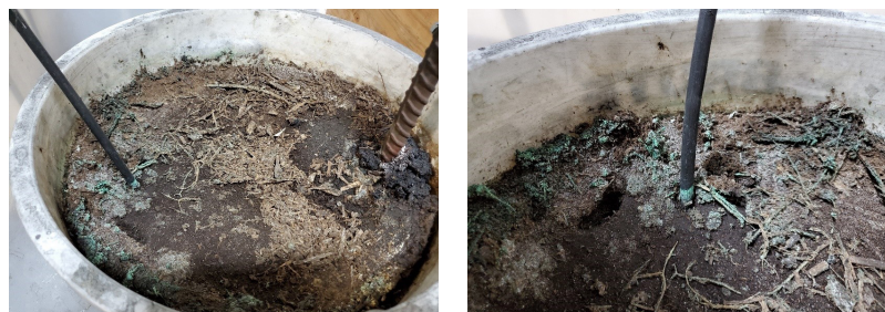
Figure 11: Blackburn GP-100 Copper Grounding Plate, After Experiment
