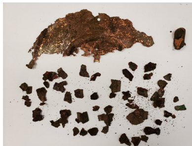
Figure 12: Blackburn GP-100 Copper Grounding Plate with Corroded Pieces Remaining in Soil, After Experiment
