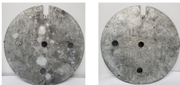
Figure 15: Galvanized Steel Plate that was Encased in ConduDisc Surround, After Experiment
