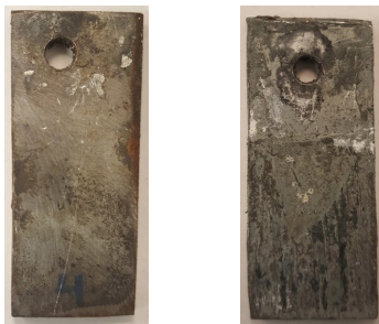
Figure 4: ConduFlow Encased Samples, Bare Steel #4 (left) and Galvanized Steel #10 (right), After Experiment
