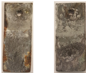
Figure 4: ConduForm Encased Samples, Bare Steel #3 (left) and Galvanized Steel #9 (right), After Experiment
