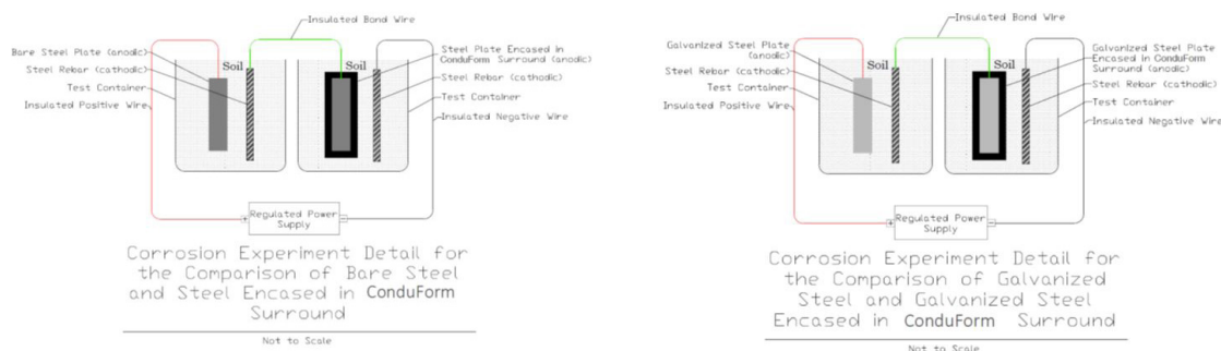
Figure 2: Schematics of the Circuit Configuration for Each Sample
