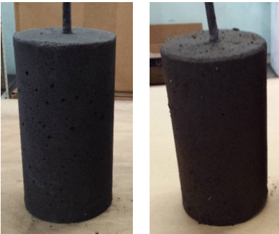
Figure 3: Copper #2 Encased in ConduForm Before (left) and After (right) Experiment
