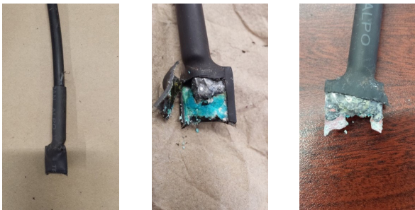
Figure 3: Copper #2 Encased in ConduForm Before (left) and After (right) Experiment
