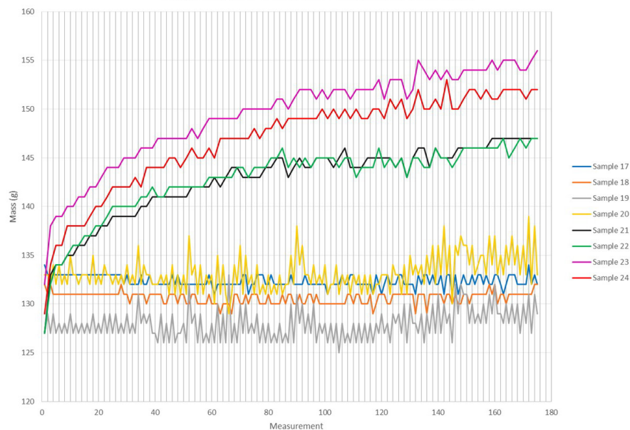
Figure 1: Changes in Mass of ConduForm Over 90 Freeze-Thaw Cycles
