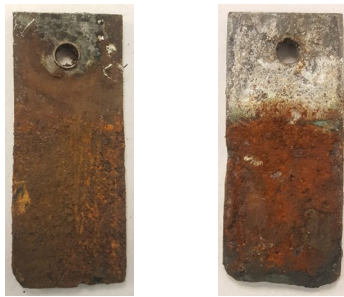
Figure 4: ConduForm Encased Samples, Bare Steel #3 (left) and Galvanized Steel #9 (right), After Experiment
