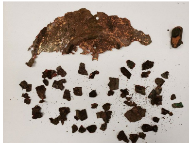
Figure 12: Blackburn GP-100 Copper Grounding Plate with Corroded Pieces Remaining in Soil, After Experiment
