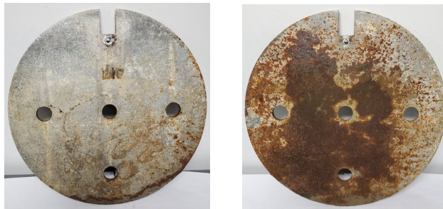
Figure 13: Galvanized Steel Grounding Plate, After Experiment
