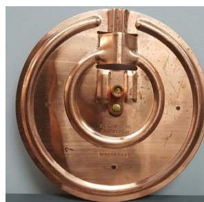
Figure 3: Blackburn GP-100 Copper Plate, Prior to the Experiment
