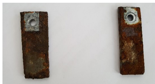
Figure 4: Uncoated Samples, Bare Steel (left) and Galvanized Steel (right), after Experiment
