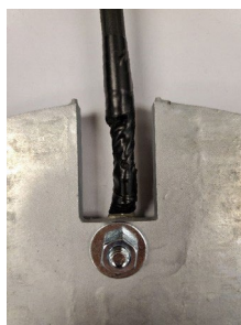
Figure 2: Copper Compression Connector Attachment to the Galvanized Steel Grounding Plate (left and middle) and the ConduDisc Inner Plate (right)
