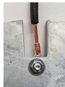
Figure 2: Copper Compression Connector Attachment to the Galvanized Steel Grounding Plate (left and middle) and the ConduDisc Inner Plate (right)
