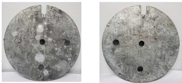
Figure 15: Galvanized Steel Plate that was Encased in ConduDisc Surround, After Experiment
