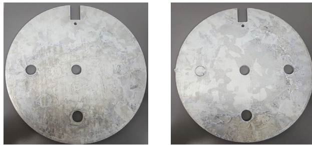
Figure 5: Galvanized Steel Grounding Plate to be Encapsulated in ConduDisc Surround Material, Prior to the Experiment
