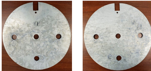
Figure 5: Galvanized Steel Grounding Plate to be Encapsulated in ConduDisc Surround Material, Prior to the Experiment
